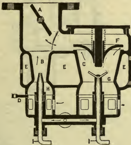
FIG. 168.—The Willet Carburetter. This consists of two carburetters in one, each with its own spray nozzle and adjustment. The small carburetter B is used for low speeds, and a second one C, cutting in on moderate and high speeds. Automatic action is secured by the spring operated valve F. The air supply of carburetter B may be regulated by valve D, having dashboard control. Closing this valve produces a strong suction on the spray nozzle in B, thus drawing a rich mixture to make easy starting possible. The valve is then opened to its normal position, which is wide open. Should the weather be cold and a richer mixture required, this valve may be closed somewhat. The entire carburetter is controlled by the butterfly throttle valve A. Nozzle H has a single opening while G is a multi-nozzle having four outlets. Both mixing chambers may be heated by the jacket E. The fuel flow to nozzle is controlled by the needle valves I.
